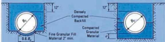
SHAPED SUBGRADE WITH GRANULAR FOUNDATION
